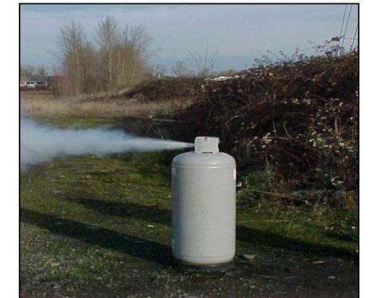
Heat has a direct effect to propane. When a container absorbs heat the liquid gas inside expands increasing pressure. Too much internal pressure can cause the *pressure relief valve* to discharge.
